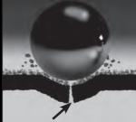
**RESULTS ON A CLASS 4 IMPACT-RESISTANT SHINGLE...** no evidence of tears, cracks, or ruptures on front or back of shingle after impact
